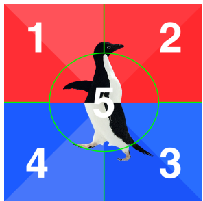
Figure 4. An example of separate regions computed for the color histogram difference measurement.
